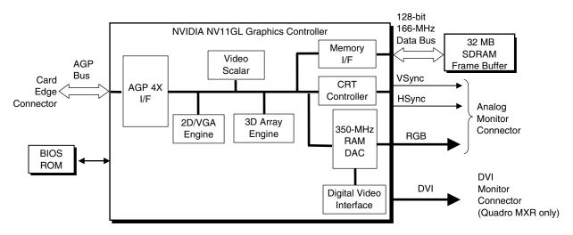
Figure E-2. NVIDIA Quadro2 EX/MXR Graphics Card Block diagram
